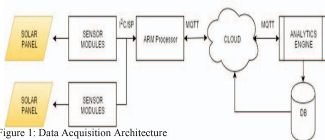
Figure 1: Data Acquisition Architecture
